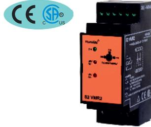
Microcontroller design, SMD Technology, Phase Failure, Unbalance, Phase Sequence, under voltage, Over Voltage, Auto reset, Fixed Unbalance setting, Fixed UV/OV settings, 2 CO output relay
