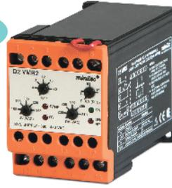
Suitable for 3 Ph-4W system, Microcontroller design, Absolute values of UV/OV settings, Phase Failure, Unbalance, Phase Sequence, under voltage, Over Voltage Neutral Fail Auto/Manual reset, Adjustable settings for Unbalance, UV/OV and trip delays, 2 CO output relay, Fixed failsafe-non-failsafe logic.
