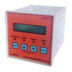
Sequencing of Booster Pumps according to the pressure switch, duty cycle is a necessity in a Booster Pump Control System. Minilec Booster Pump Controller fulfils all the requirements of a Booster Pump Control Panel. Suitable for 2/3 Pumps or 4/5 Pumps. F3 BPC1 is suitable for 2/3 pumps and F5 BPC1 is suitable for 4/5 pumps, operates on  $90\text{-}270\,\text{V}$  AC/DC supply and has RS 485 output port.
